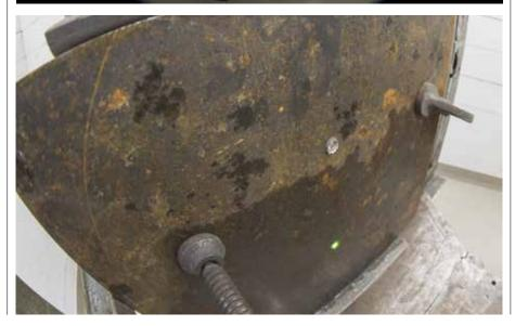
Our test firing at Wiltshire Ballistic Services was a clear demonstration of the lack of protection a 7mm-thick mild steel plate offers against a 7.62mm AK47 round.
